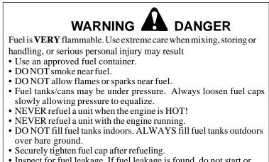
• Inspect for fuel leakage. If fuel leakage is found, do not start or operate unit until leakage is repaired.
